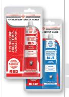
SILICONE GASKET MAKER is one component, ready to use sealant designed for form-in-place gasketing where high temperature occur. ASMACO RTV Silicone Gasket Maker cures upon contact with atmospheric moisture at room temperature to form an elastomeric, resilient silicone rubber gasket. The rubber-like seal formed after curing is highly resistant to weathering and UV exposure, is unaffected to high and low tempera-
